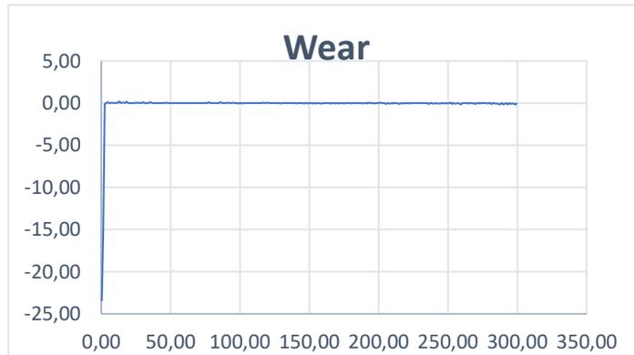
Gambar 3.16 grafik wear 1 lapisan coating percobaan pertama.
